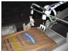
Invisible adhesive is applied to a flour bag at Rocky Mountain Flour Milling LLC, in Platteville, CO.
